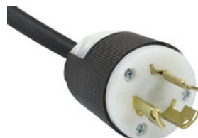
L6-15 Twist Lock Plug 15 Amp / 250 V Rated
