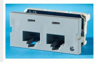
Clarity 6 Series II module two jack ports (1 unit), ETL verified to TIA Category 6 component specification. Front-loading and front removable. New universal T568A/B wiring label and tapered wiring towers simplify termination. Center tuned to Clarity 6 patch cords for optimum performance.
