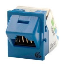
Clarity 6 Angled TracJack, ETL verified to TIA Category 6 component specification, is front-loading and front removable. New universal T568A/B wiring label and tapered wiring towers simplify termination. Center tuned to Clarity 6 patch cords for optimum performance.
