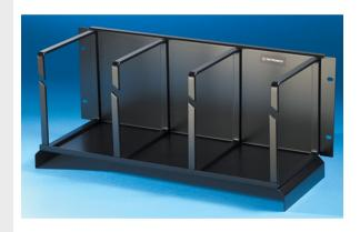
Ortronics bend limiting cable management panels have curved falls that protect against cable crimping and also maintain proper bend radius. The panels are ideal at the top of standard 19" EIA racks. 7" H x 7" D rings with waterfall, 8.34" H x 19" W, 4 rack units, black.
