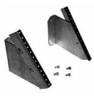
Swiveling rack angles drop 45 degrees to provide convenient access to equipment mounted on patch panels. Provide additional patch panel location in 36- and 48-in. (914- and 1219-mm) high cabinets. Made of self-grounding, plated 12 gauge steel. Mounting hardware included. Set of two.
