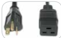
010-9335: 5-20P to C19 125V, 20A straight blade 8-foot, 12 AWG/3-wire
