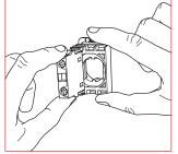
The contact blocks/lamp block are then snapped on to the holder...
