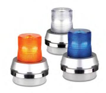
The 51XBR superbright LED signal is a combination audible and visual signal providing two levels of sensory notification. The integrated horn is synchronized with the flashing LED. The units are designed for indoor or outdoor applications and are available in 24V DC or 120V AC. The polycarbonate double fresnel lens is designed to magnify the superbright LED inside, while maintaining a high level of scratch and impact resistance.
