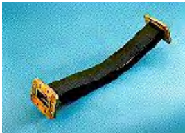
F034KKS4 FlexTwist™ Flexible Twist for WR34, 22.0–33.0 GHz, with interface types PBR260 and PBR260, 1000 mm
