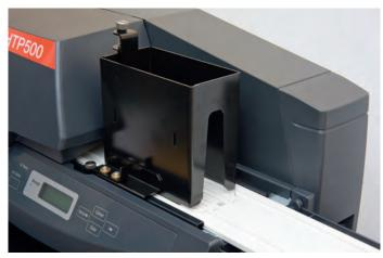
The feeder allows printing of series of markers. It can be loaded with up to 64 marker cards.
