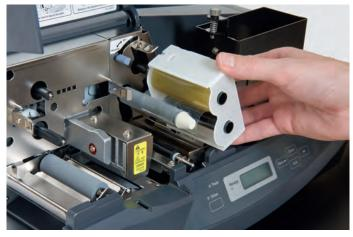
The HTP500 V2 printer is equipped with a cleaning tape. It cleans the media before printing to ensure best printing quality.
