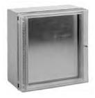
Clear molded polycarbonate window has a 31.8-mm (1.25-in.) clear space between enclosure front opening and window surface. Space also accommodates equipment mounted on optional front plate. Window kit is hinged on left side with a 140-degree door opening and a quarter-turn slotted latch. Includes mounting hardware for window and optional front plate. Die-cast backing plate has a black polyester powder finish. This kit can be used as an accessory window kit on other Hoffman enclosures.
