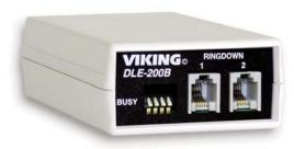
The **DLE-200B** Line Simulator produces two way communication between standard telecom products such as modems, fax machines, Key Systems, PABX's and standard single line telephones. The Line Simulator can also provide sales people with a cost effective, easy to use method of conducting on site demonstrations, eliminating the need to locate phone lines and disrupt the customer's phone service.
