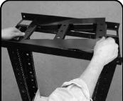
Place cable tray on top of rack between upper rack support brackets and press tray into
