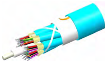
760004465 | R-036-DS-8W-FMUYL Riser Distribution Cable, 36 fiber multi-unit with 12 fiber subunits
