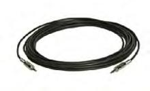
Kramer's CP-A35M/A35M series mini stereo audio cables are premium quality plenum rated cables constructed of shielded pair style cable terminated with precision male tip-ring-sleeve style 3.5mm connectors at each end. They offer outstanding durability and high performance for any stereo unbalanced audio signal application where a plenum rating is required.
