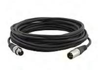
Kramer's XLQ cables are quad style professional-grade mic or line level audio cables. 4-core star quad cables with mutually offsetting twisting technology can reduce induction noise levels to 10% of that in regular two-pair balanced microphone cable.
