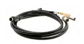
Kramer's s-Video (Y/C) breakout cable is constructed of dual mini coax cables with a male s-Video (4-pin) connector on one end and 2 BNCs on the other. They are used for converting an s-Video signal from the typical 4-pin format to higher quality dual BNC format preferred for long cable runs.
