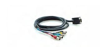
Kramer's computer graphics video breakout cables are constructed of 5 mini coax cables with a molded 15-pin HD (M or F) on one end and 5 BNC (M or F) on the other. They convert between the two most common cabling formats used for routing computer graphic video signals, 15-pin HD, and 5 BNC.
