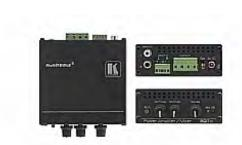
The 907xl is a high-performance power amplifier for line-level stereo audio signals. It accepts a balanced stereo audio signal on a terminal block connector and an unbalanced stereo signal on RCA connectors. It delivers 40 watts per channel into an  $8\Omega$  load.
