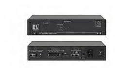
The Kramer 914 is a high-performance 2x100W power amplifier that accepts a balanced stereo audio input on a 5-pin terminal block and converts the signal into a differential stereo audio output for speakers on a 4-pin terminal block.
