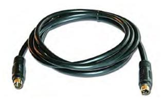
Kramer's SM series cables are high performance s-Video (Y/C) cables with molded 4-pin mini DIN connectors at each end. Luminance and chrominance signals are carried on separate internal coaxes for superior quality over composite video.
