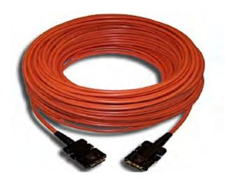
Kramer's all DVI cable system is constructed of high-performance hybrid cable containing fiber optic and copper wires terminated with DVI-D connectors on each end. They are designed to transmit DVI-D signals extremely long distances with pristine digital image quality video with the copper cable carrying additional data required for HDCP compliance.
