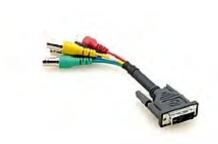
Kramer's ADC-DMA/5BF-1 is a short adapter cable designed to adapt between the analog pins of DVI-I and typical RGBHV. DVI video cards often output signals in both digital and analog format and, conversely, display devices often accept an analog VGA type signal using a DVI connector.
