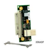
The IONADP is an adapter card that allows the ION Platform chassis to be backwards compatible with Point System™ modules. This adapter is designed to sit between a Point System™ module and the backplane of the ION chassis. The purpose of the IONADP is to lengthen the Point System™ module so it can be securely mounted in an ION chassis while also connecting to the backplane allowing the ION chassis to power the Point System™ module.
