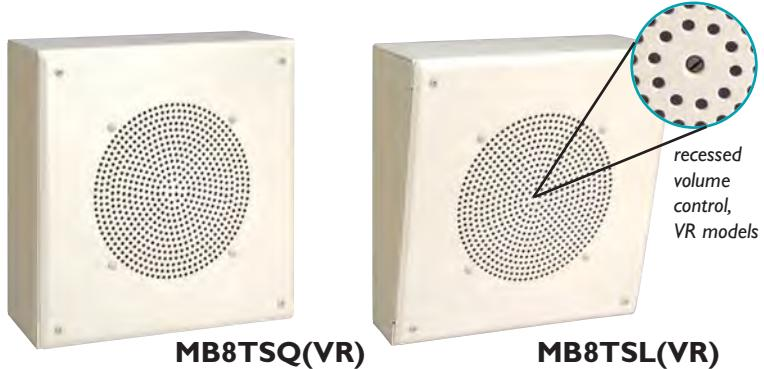
**Description** Bogen's MB8TSQ and MB8TSL speakers feature an all-steel surface-mounted enclosure with an 8" cone loudspeaker and multi-tap 4-watt 70V/25V transformer. The MB8TSQ speakers are suitable for ceiling or wall mounting. The MB8TSL speakers are designed primarily for wall mounting, with front face angled downward by 12.5 degrees. Models with VR suffix have a recessed volume control at the center of the grille (see *inset*).
