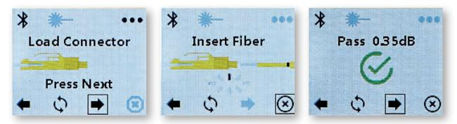
Guides the user through the termination process with simple step-by-step prompts and on-screen visuals. Ensures the field fiber and fiber stub are in proper alignment before camming.
