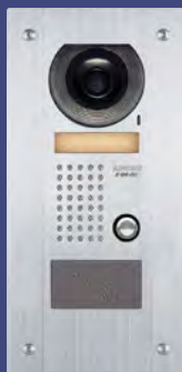
JF-DVF-HID Card Access Video Door Station • HID® ProxPoint® Plus Proximity Card Reader • Fixed camera • Stainless steel • Flush mount H: 11-5/8" W: 5-3/4" D: 1-7/8"
