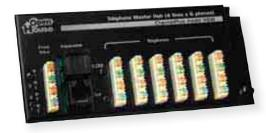
The Model H616 Telephone Master Hub provides a superior method of telephone distribution for structured wiring systems. The Model H616 distributes up to four telephone lines to up to six telephone wall plates. An RJ-31X jack is provided for security system connection. Additionally, the Model H616 includes an RJ-45 jack for telephone line expansion.
