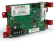
FCB-1000/RM Fire Communication Bridge (Optional rack mount enclosure) Connect 1 to each P-Link Circuit
