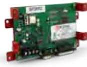
SPG-1000/RM Serial Parallel Gateway (Optional rack mount enclosure) Connect up to 31 to each P-Link Circuit
