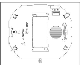
Switch positions 1 and 2 in the down position to select isolated horn and strobe power inputs. Switch 3 selects between temporal or non-temporal tone. Up is temporal. Switch 4 selects between mechanical or high frequency tone. Up is mechanical. Switch 5 selects between high or low dBA. Up is high dBA.
