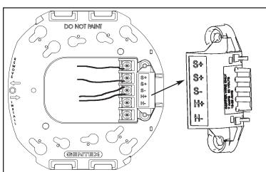
The access holes are provided in the back of the terminal block to allow the voltage to be measured directly without removing the device. Typically this would be done at the end of the line to confirm design criteria. Most measurements will be taken using the S+ and S- locations although access is provided to other locations. *NOTICE:* CARE SHOULD BE TAKEN TO NOT SHORT THE TEST PROBES.
