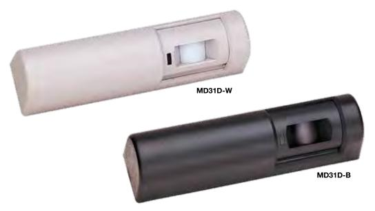
The SDC MD31D Passive Infrared Detector is specifically designed for request-to-exit applications. The coverage field is internally pointable. When angled 14° down, coverage may be 5 x 6 feet at 7 feet high to 10 x 12 feet at 15 feet high. The MD31D projects a wrap around "U" pattern down and away from the door to inhibit tampering.
