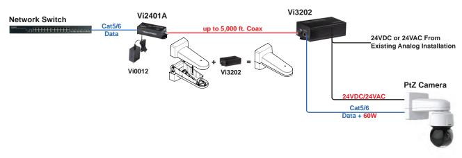
PTZ Camera is powered by PoE and its Heater/Blower powered by existing 24VDC or 24VAC power supply.
