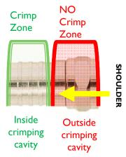
4) When crimping the connector, only crimp the areas below the shoulder ring.
