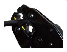
5) Place assembly in appropriate crimp tool cavity (30-503 shown) and crimp.
