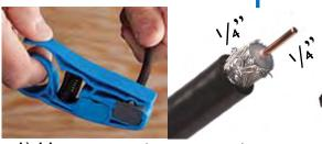
I) Use coax stripper to strip cable so '4" of conductor and '4" of braiding are exposed. (45-605 shown)
