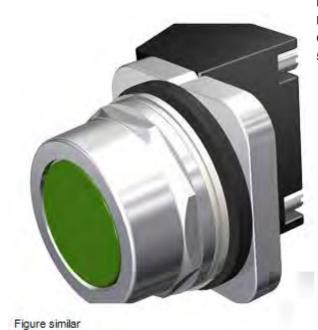
30mm Command/52, Chrome Finish Heavy Duty, Watertight/Oiltight Point-of-Purchase Kit Pushbutton Non-Illuminated Flush Button Plastic Cap 1ea.: Green, Black, Red, Yellow, Blue 2 Position Momentary with 1 N.O. Heavy Duty Contacts, A600/P600 UL Listed, CSA Certified NEMA 1,3,3R,4,4X,12,13 & Automotive Standards 1 52NL03 (START) and 1 52NL11 (ON) Legend Plate
