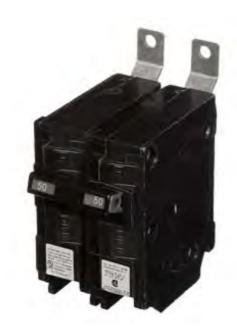
Siemens Low Voltage Molded Case Circuit Breakers Panelboard Mounting 240V Circuit Breakers - Type BL, 2-Pole, 120/240VAC are Circuit Protection Molded Case Circuit Breakers. Type: BLH Application: Electrical Distribution Standard: UL 489 Voltage Rating: 120/240V Amperage Rating: 50A Trip Range: Thermal Magnetic Interrupt Rating: 22 AIC Number Of Poles: 2P
