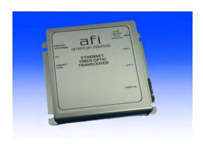
The American Fibertek 48-PoE Series transmits and receives (2) copper 10/100/1000 Base-T Ethernet signals at the RJ45 ports and (1) optical 1000 Base-X over 1 or 2 multimode fibers. The system is comprised of two units forming a point-to-point communications link.
