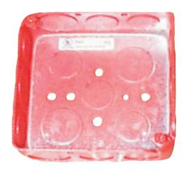
A steel back box painted red and measuring 8.6 cm (3.375 in.) square by 5.6 cm (2.1875 in.) deep. It has knockouts for interior surface mounting, concealed conduit mounting, or semi-flush mounting applications.
