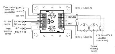
The E-2WIRE can be set for Class B or Class A operation using the slide switch located on the front of the module.
