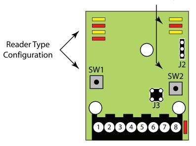
5VDC - 12 VDC Reader Power Jumper
