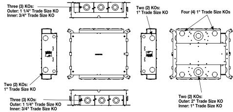
NOTE: Three (3) removable knockout plates per side allow for the EFB6S-2HUB 2" conduit adapter to be installed.
