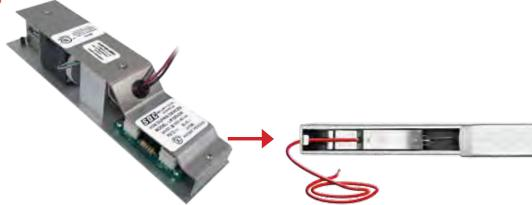
The SDC LR100 Series Electric Latch Retraction Kit enables electric access control and dogging of mechanical exit devices. When energized the motor retracts the exit device latch and pulls the pushpad into the dogged (depressed) position enabling momentary or sustained push and pull operation of the door.
