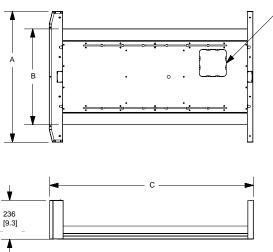
6 1/2" x 6 1/2" (165mm x 165mm) knockout compatible with Cool Boot® p/n: CTGN6X6 or cable bezel p/n CTNBZC6X6
