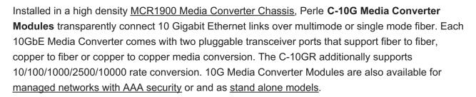
Fiber to Fiber and Copper to Fiber conversion is achieved by inserting XFP or SFP+ fiber transceivers that support multimode and single-mode fiber, including CWDM/DWDM wavelengths. Copper to copper is achieved by inserting SFP+ Direct Attach Cable (DAC), also known as twinax, or XFP 10Gbase-CX4 transceivers.
