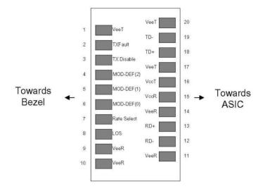
Pin-out of connector Block on Host board
