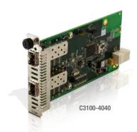
The ION C3100 is a fiber to fiber media converter module. It is protocol independent and supports data rates from 100Mbps to 2.5Gbps through two open SFP slots. This any-rate to same-rate converter can be used to perform reliable and cost-effective single mode to multimode fiber conversion or it can be used to provide wavelength conversion in CWDM applications. The ION C3100 is a manageable device when installed in a managed ION chassis.
