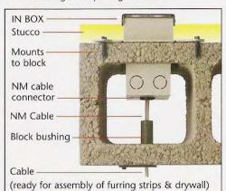
Cutaway showing IN BOX and plastic block bushing mounted in masonry block.
