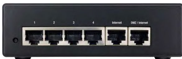
Figure 2. Back Panel of the Cisco RV042G
