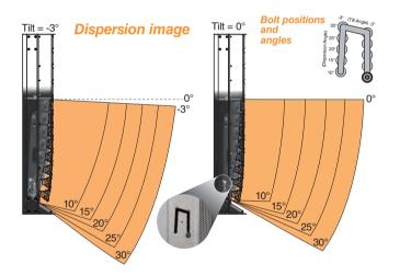
The system provides uniform sound output with little attenuation over distance and permits operators to combine speakers freely to suit the conditions. Together, these features ensure the clear audibility required by houses of worship, auditoriums, airports and other venues with complex acoustic conditions. With its slim styling and availability in a choice of two colors, the system also blends in seamlessly with virtually any interior décor.
