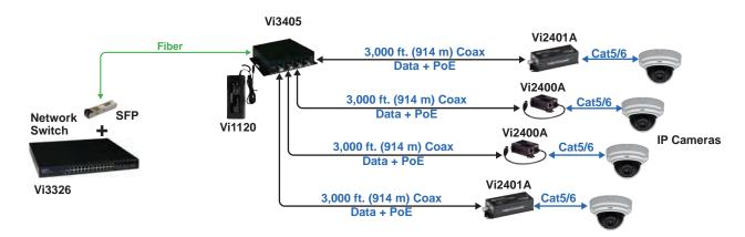
Up/down links can use either the 100Base-T port or Fiber port for distances up to 80Km.
