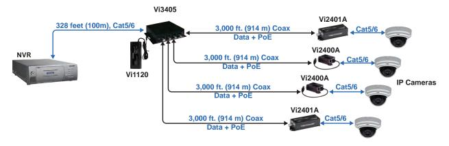
For smaller systems direct connection from Vi3405 to NVR or Computer running VMS can eliminate the need for an extra network switch when converting from analog to IP video.
