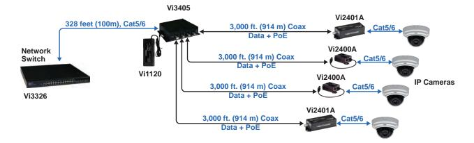
Vi3405 provides a simple method to convert existing analog systems to IP Video.
