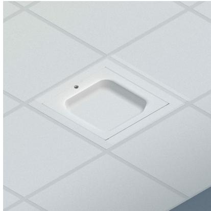
This locking retrofit door is designed to provide a convenient way to mount and secure APs in 1047 Series AP enclosures. To remove the old door, simply unlock the door, open the door to a 90° angle, align the tabs of the door mount to the slots in the back-box hinge opening, and slide the door forward. Simplify equipment replacement without lifting ceiling tiles.
